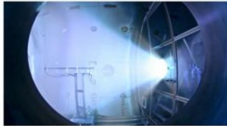
Fig. 4.4 The VX-200 plasma under high power operation
