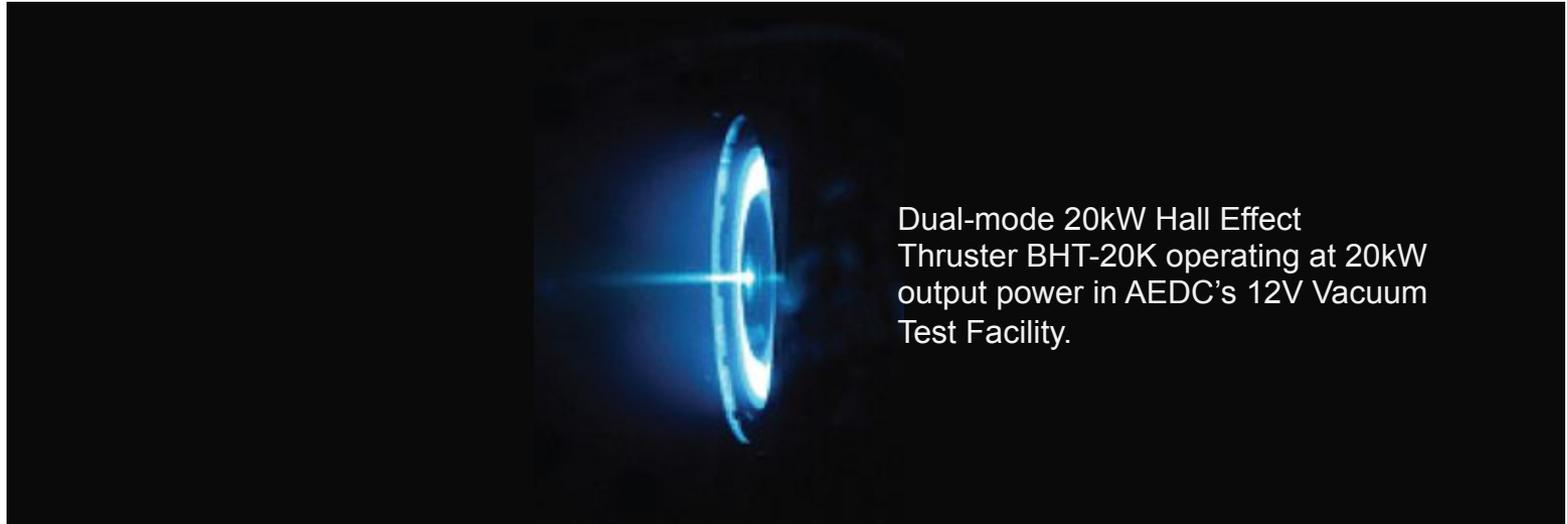
Dual-mode 20kW Hall Effect Thruster BHT-20K operating at 20kW output power in AEDC's 12V Vacuum Test Facility.
