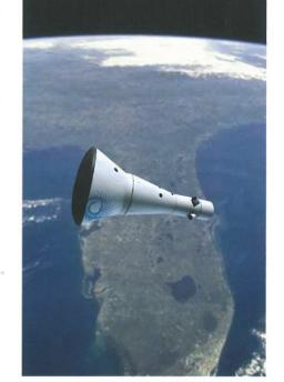
The Almaz collection of pressurized and unpressurized sections can be tailored to the widest variety of possible missions, from short duration (30 hr) orbital flight to circumlunar missions lasting a week. Both pressurized RRV and space station module are flight tested and qualified for long duration missions.
